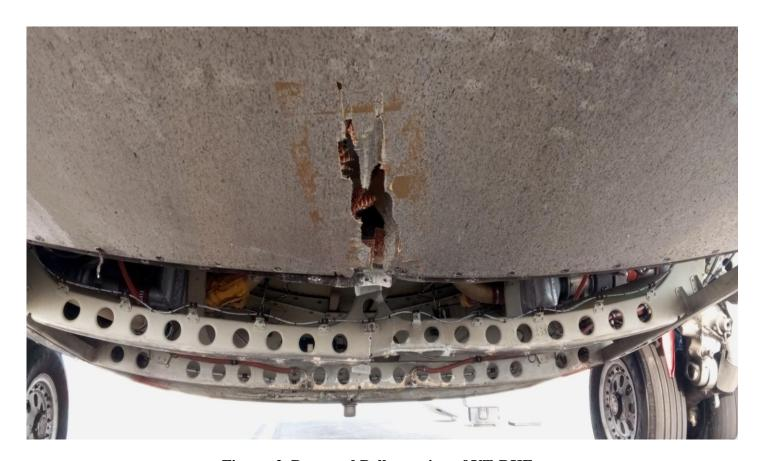
Figure 2. Damaged Belly portion of VT-RKF
